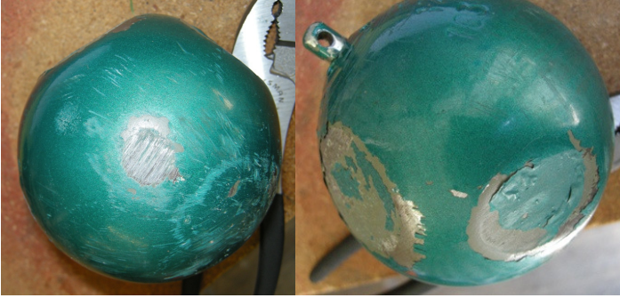
Damaged hammer head
